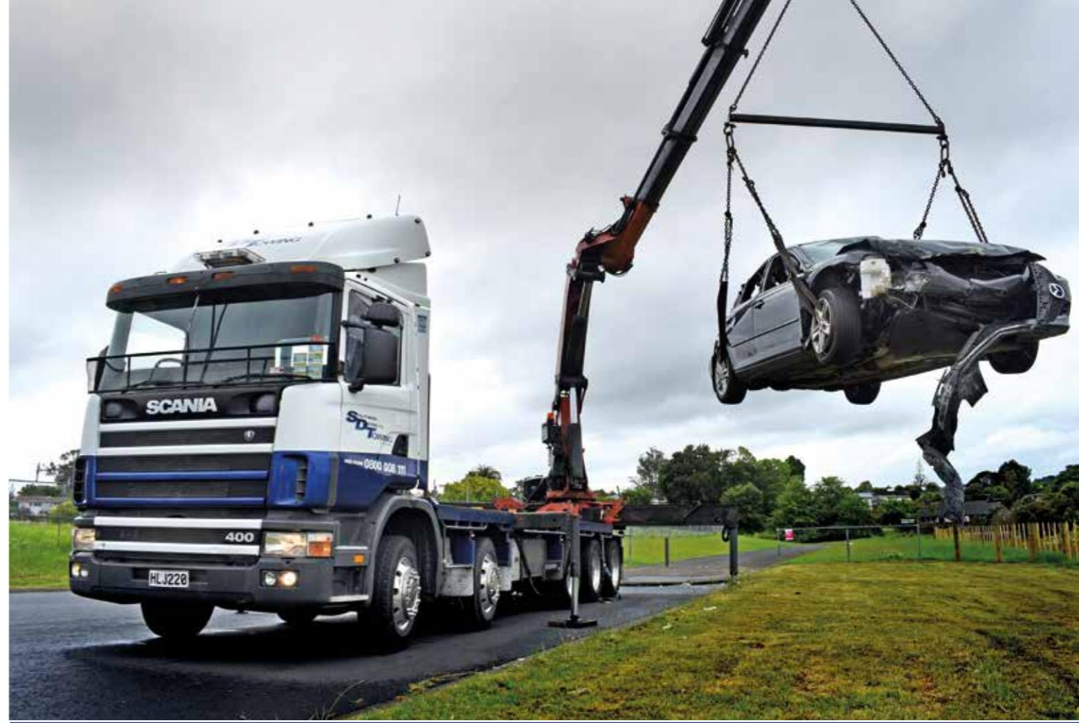
Scania 400 10x4 Hiab unit, capable of lifting up to 12 tonnes close in, recovers a wreck
